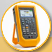
With the new 729 Automatic Pressure Calibrator, generating and controlling pressure for each test point is as simple as pressing a button. Simply input the calibration starting and ending pressures, and the desired number of set points, and the calibrator does the rest—all with out hand pumps, or manual fine adjustments.
