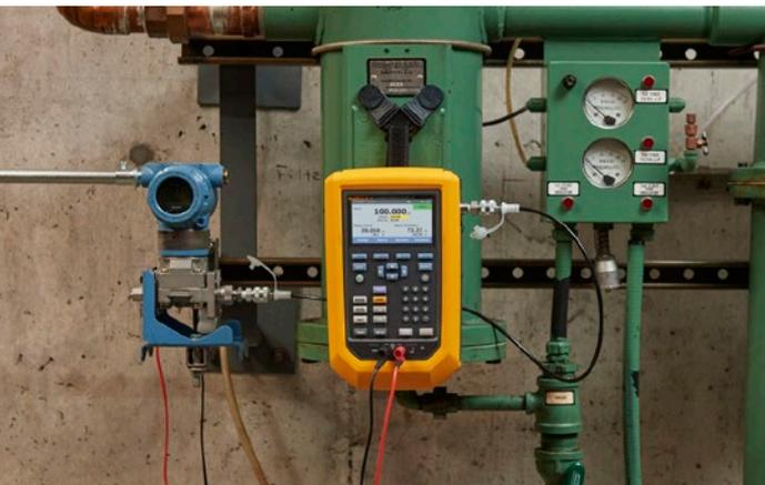
“The automatic pump on the 729 pressure calibrator reduces hand pump instrument error as well as reducing calibration time by about 40 %.”
