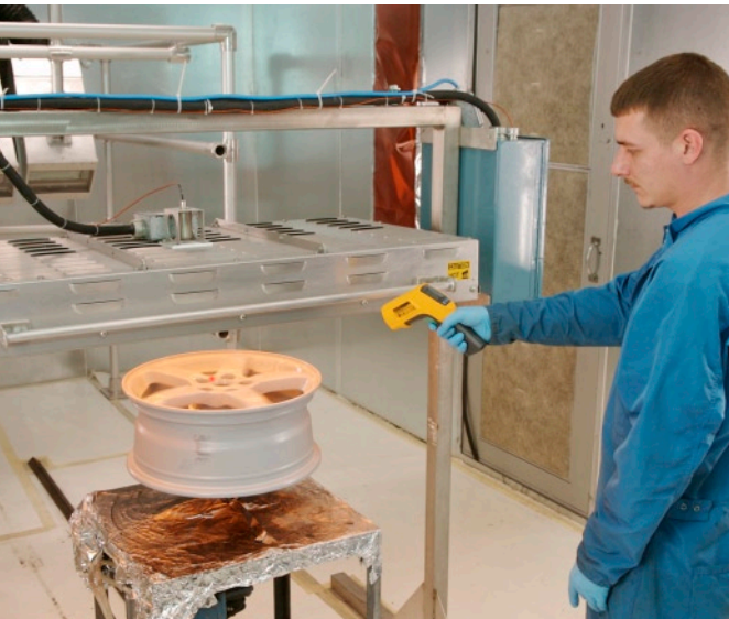
James Solomon monitors the surface temperature of a wheel that just had a primer coat applied in the spray booth in Helios Coatings research lab.
