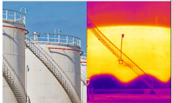
Thermal imaging technology can help oil and gas companies gauge tank levels without direct contact, as well as distinguish small changes in temperature between liquids or solids of varying densities and specific heat characteristics.
