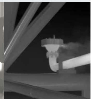
Optical Gas Imaging can help users detect and locate fugitive gas leaks early to avoid a potential platform shutdown.
