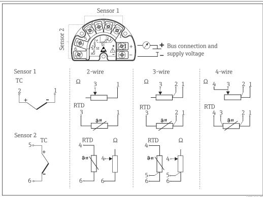
**₽** 2 Wiring the transmitter
