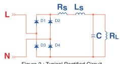
Figure 2 : Typical Rectified Circuit
