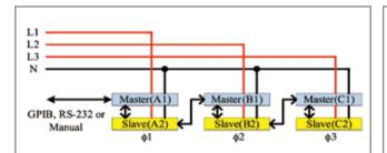
Figure 11: Parallel/3-Phase Y connection
