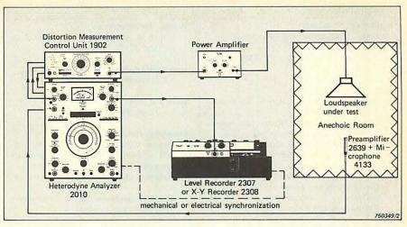
Fig.10. Set-up for recording the distortion characteristics of a loudspeaker
