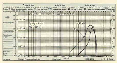
Fig.9. Difference-frequency analysis recorded with the set-up in Fig.8
