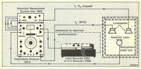
Fig.11. Set-up for recording intermodulation and difference-frequency distortion analyses of a microphone
