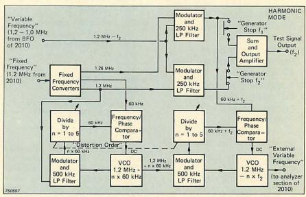
Fig.2. Simplified block diagram of the 1902 in the "Harmonic" mode
