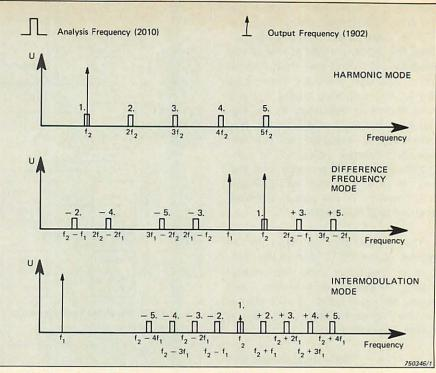
Fig.5. Relative position of analysis frequencies of 2010, and test signal frequencies of 1902 in the three different modes of operation
