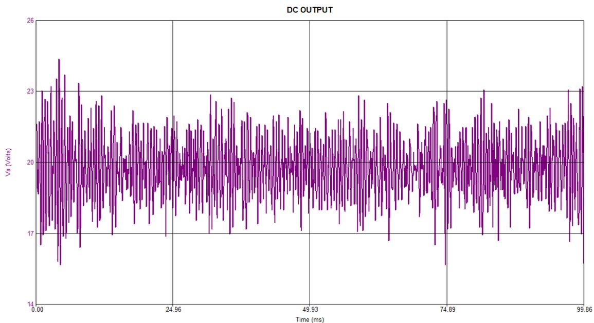
This output goes through an inverter in order to convert the DC to AC. An unconditioned AC voltage can create various power quality issues.
