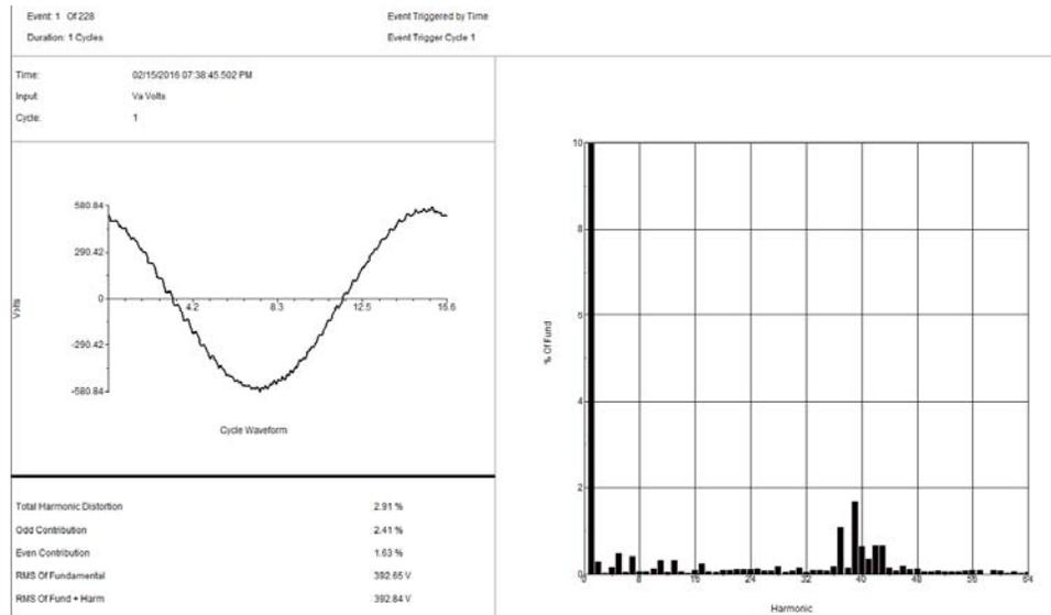
Higher frequency harmonics increase heating effects in wires and coils.
