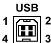
Figure 3-4: USB Connector pin orientation.
