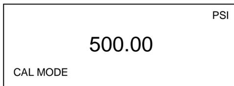
Use the Pressure Standard to output 500.00 psi (100%). After the output has stabilized, press the ENTER key to continue. As the unit takes readings, the screen will show ----- . When the readings are complete the screen should look as shown in the illustration that follows.
