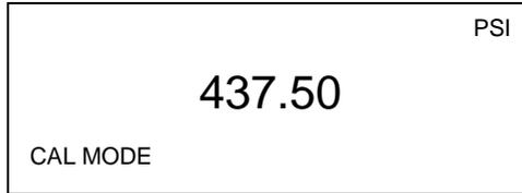
Use the Pressure Standard to output 437.50 psi (87.5%). After the output has stabilized, press the ENTER key to continue. As the unit takes readings, the screen will show ----- . When the readings are complete the screen should look as shown below.
