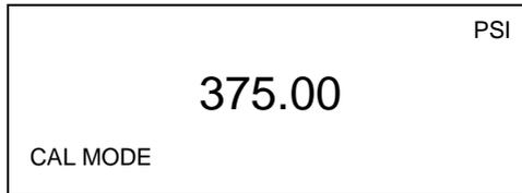
Use the Pressure Standard to output 375.00 psi (75%). After the output has stabilized, press the ENTER key to continue. As the unit takes readings, the screen will show ----- . When the readings are complete the screen should look as shown below.
