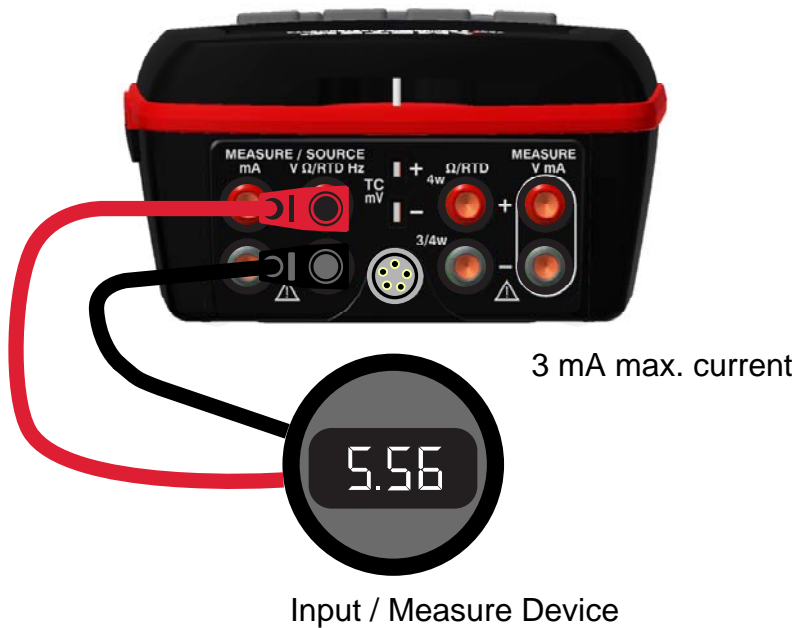
Figure 18 Connections for Testing an Output Device
