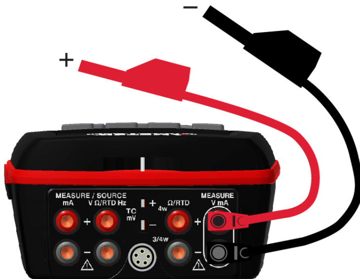
Figure 13 mA current measurement connection (upper window)
