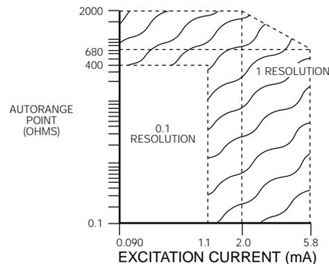
Note: Above ranges are for READ mode in which the Model 211 provides a 1 mA excitation current. SIMULATE mode operates in these ranges with external excitation currents between 0.090 and 1.1 mA. Resolution will be 1°, or 0.10Ω, in all ranges for excitation currents between 1.1 and 5.8mA
