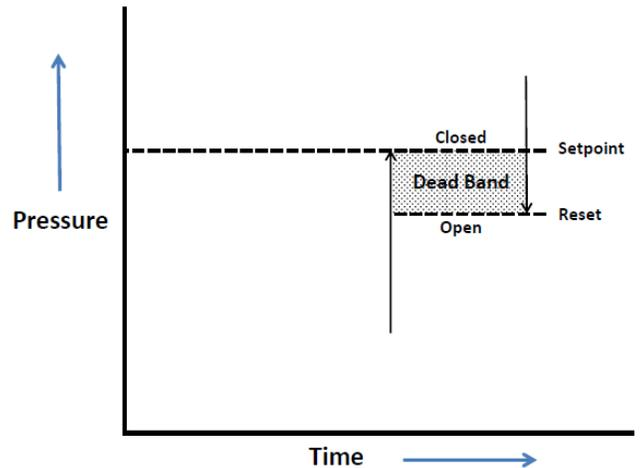
The application of the switch will largely determine which functions need to be calibrated. For the purpose of this application note, we will assume the tolerance, repeatability, and dead band need to be calibrated for a single-point switch. To illustrate the calibration, we will use the following switch specifications:
