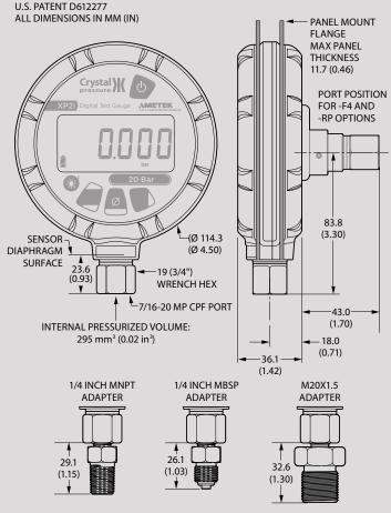
ADDITIONAL SENSOR LENGTH WITH OPTIONAL FITTING ADAPTERS
