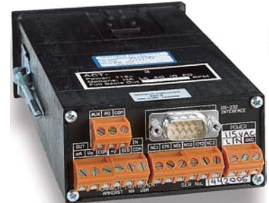
ACT-3 Panel Tachometer/Ratemeter/Totalizer
