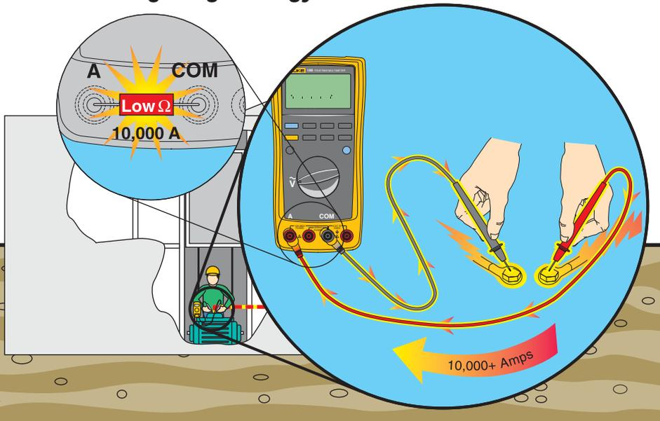
Figure 3. Misuse of DMM in Ammeter Mode.
