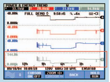
With the demand interval set correctly, the Fluke 430 Series will plot one average demand reading for each demand interval. Your peak demand will be the highest of these readings.
