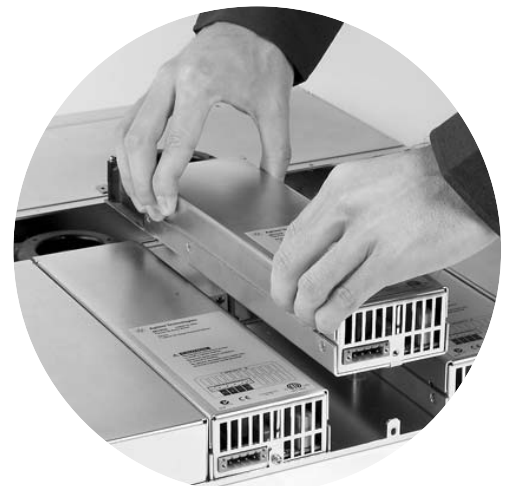
Figure 6b. User re-configurable modular system
