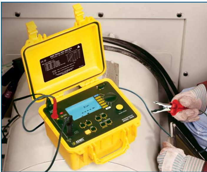
Model 5060 performing insulation test on a generator.
