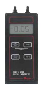
Ideal for field or laboratory use, the Model 476A Single Pressure Digital Manometer measures low pressures from -20 to 20" w.c. with ±1.5% full scale accuracy. Designed especially for the HVAC contractor, the Model 476A can be used to set supply pressures, verify pressure switch operation, adjust regulators, check pneumatic systems and computer peripherals. The rugged, handheld unit is constructed with an extruded aluminum case for exceptional durability.
