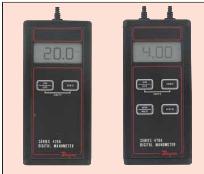
**Ideal for field or laboratory use**, the Model 476A Single Pressure Digital Manometer measures low pressures from -20 to 20" w.c. with  $\pm 1.5\%$  full scale accuracy. Designed especially for the HVAC contractor, the Model 476A can be used to set supply pressures, verify pressure switch operation, adjust regulators, check pneumatic systems and computer peripherals. The rugged, handheld unit is constructed with an extruded aluminum case for exceptional durability.
