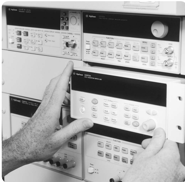
Low-cost switching system for automated testing
