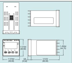
Monitor and control temperature or process applications with precision using the Series 16B controllers. The units offer two separate outputs for dual loop control in direct or reverse acting. Select relay,
