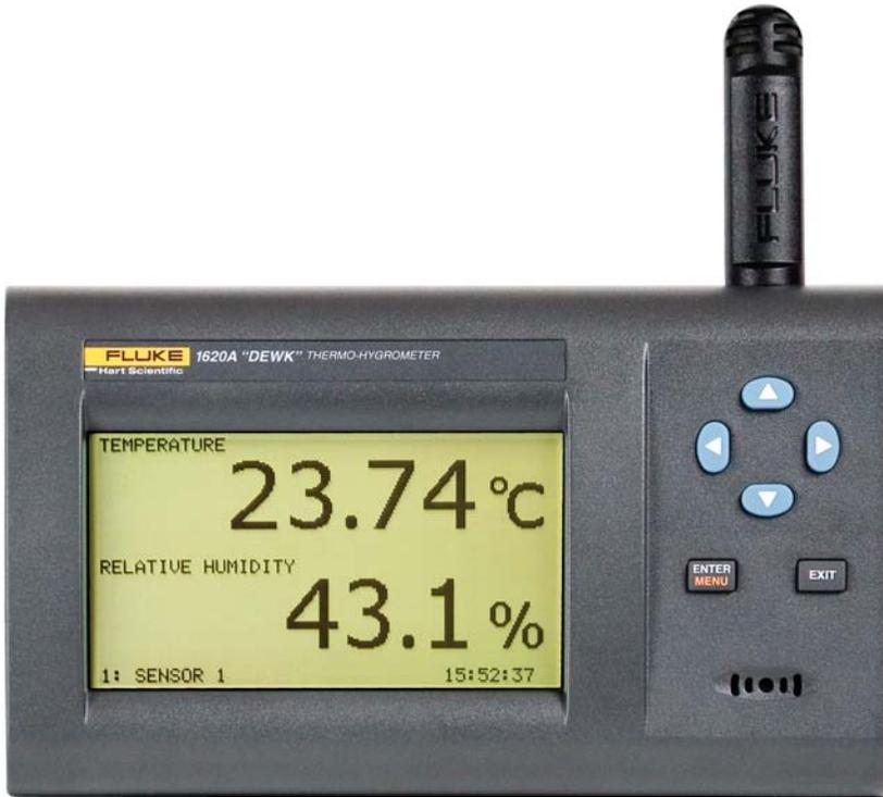
35 °C. Relative humidity readings are to  $\pm 2$  %RH from 20 %RH to 70 %RH.
