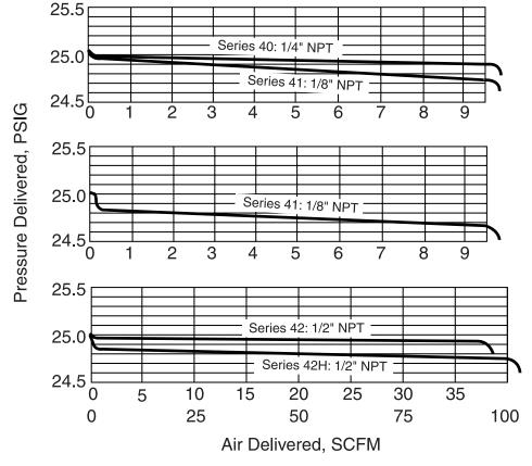
**Test Procedure:** Each 30-psig-range regulator was adjusted to 25 psig with 100 psig supply and no flow. Flow was increased to maximum capacity. All regulated pressure readings were taken at gauge connection in the body of the regulator.
