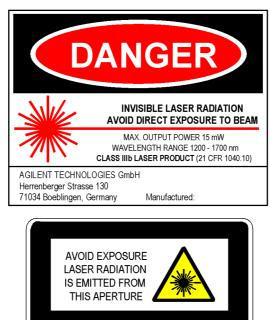
Figure 1 USA Safety Labels (81480A, 81680A, 81640A, 81682A, 81642A, 81689A)
