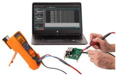
Utilize the U5404A remote switch probe to measure, save and send measurement readings over to Keysight handheld meter logger software with just a press of the button.
