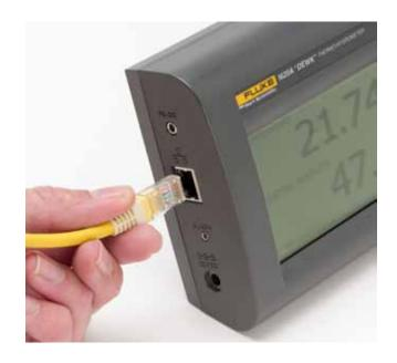
disconnected from the base unit (the display), and freshly calibrated replacements are reconnected in their place. Only the sensor modules need to be returned for calibration. In fact, it's the accredited calibration of these sensors that is responsible for the high accuracy of the DewK.
