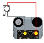
Figure 2-18 Measure current on CH1. Range ± 55 mA
