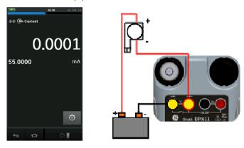
Figure 2-20 Measure current with external loop power (Range: ±55mA)
