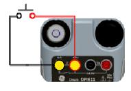
Figure 2-22 Switch Test
