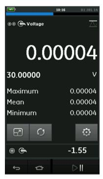
Figure 2-12 Max/Min Example
