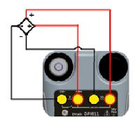
Figure 2-23 Measure DC Volts (10V) or DC mV (10V) on CH1
