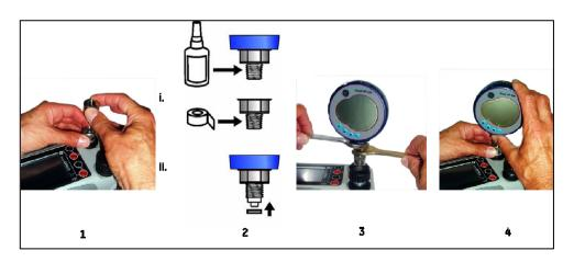
Figure 2-4 Attach / Remove Pressure connections
