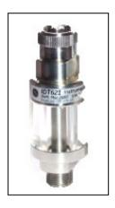
It prevents contamination of the DPI611 pneumatic system and cross contamination from one device under test to another. The trap connects directly to the pressure port and replicates the DPI611 quick fit connection for compatibility with standard adaptors, adaptor kits and hoses
