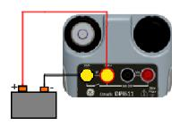
Figure 2-19 Measure DC Volts or DC mV on CH1.
