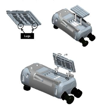
Figure 1-1 Battery Cover Insert
