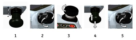
Figure 2-5 Vacuum or Pressure operation
