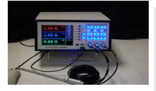
The Model 8030 three channel GAUSS TESLA METER from F.W. Bell leads the way for Advanced Hall Effect Magnetic measurement technology. The easy to use front panel programming feature incorporates the latest in user control operations. The 8030 is capable of measuring and displaying seven different parameters per channel – flux density, frequency, temperature, min, max, peak and valley. With the 8030's vector summation feature, that makes a total of 27 different parameters.
