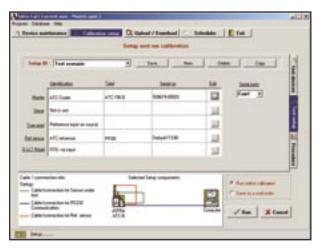
The JOFRACAL calibration software supports automatic calibration for all JOFRA dry-block calibrators equipped with an RS232 serial data interface including the JOFRA DTI-1000 digital thermometer. For semi-automatic calibrations, the software also supports liquid baths, ice points, or other dry-block heating and cooling sources. Using the software's "SCENARIO" function allows for combining instruments in virtually any configuration.
