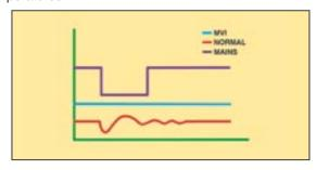
The JOFRA ATC series calibrators ATC-250, -320 and -650 employ the MVI, thus avoiding such stability problems. The MVI circuitry continuously monitors the supply voltage and ensures a constant energy flow to the heating elements. All other ATC models run on stabilized DC voltage and thus do not need the MVI circuitry.
