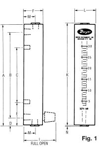
Dwver Visi-Float<sup>®</sup> Series Flowmeters are furnished in two models (see Figure 1) each available in a broad choice of flow ranges with direct reading scales for air, gas or water. Installation, operation and maintenance are very simple and only a few common sense precautions must be observed to assure long, trouble-free service.
