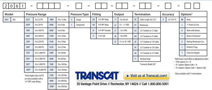
Ordering Example: 2061025PG2M11048CN - Model 206, 0 to 25 PSIG, Gauge pressure, 1/4" NPT Male fitting, 4 to 20 mA output, 4' Cable Length, ±0.13% FS Accuracy, 11 Point Cal Cert option
