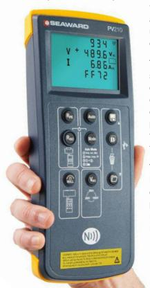
that it can be transferred to the PVMobile app alongside the rest of the test data. PVMobile can be used to convert measured data to STC for comparison with manufacturer's published data.
