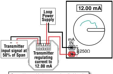
Control loop with the transmitter limiting the current to 12.00 mA.
