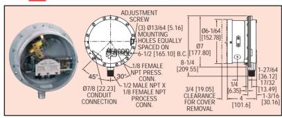
**Large diaphragm sensitivity** and time proven dependable design are combined in model PG differential pressure switches. Visible dial reduces "start up" time and helps prevent calibration errors. External adjustment allows set point change without removal of cover. Unit is listed by UL, FM and CSA.
