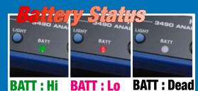
Be well-informed about the condition of your batteries. Green signals that the battery level is sufficiently high, and red warns of low battery power. Replace the batteries before the LED turns completely off.
