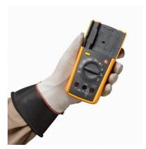
The New Fluke 233 Remote Display Digital Multimeter
