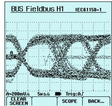
**Figure 9:** A Fluke 125 screen showing a cluttered and noisy signal.
