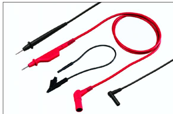
**Figure 2:** The STL120 (red) and TL75 (black) test leads are the primary tools for making test connections onto a FOUNDATION Fieldbus. When encountering heavy noise on the bus, try the shorter lead with the alligator clip (center item). All three items are standard with the Fluke 125 Scopemeter.
