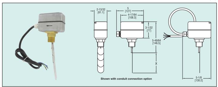
The Series FS-2 Vane Flow Switch offers an economical flow proving solution. Custom set points tailored for the application are enabled by field adjustable vane layers and a set point adjustment screw. The FS-2 features an aluminum weatherproof housing for outdoor installation. Paddles are adjustable to fit 1" to 8" size pipe. FS-2 is ideal for use in "flow or no flow" applications in cold and hot water systems. Perfect for proving flow in boilers, hot water heaters, and chillers.
