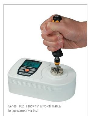
Series TT02 Torque Tool Testers present a simple and accurate solution for testing manual, electric, and pneumatic torque screwdrivers, wrenches, and other tools. These testers are compact and rugged, suitable for production environments. A universal 3/8" square receptacle accepts common bits and attachments. The TT02 captures peak torque in both measurement directions, and also calculates 1st and 2nd peaks, useful for click-type tools.
