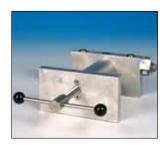
System D is an easy-to-use calibration system. Place the pump on a flat surface and turn the handle to generate pressure. You can adjust the calibrator to fit the best viewing angle. The system includes a manifold for connection of the test device, a fine adjustment vernier valve (optional), and a reservoir for extra oil or water (optional).
