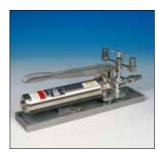
The system includes a manifold for connection of two test devices and the fine adjustment vernier valve is standard. The System F comes in a aluminium carrying case with cutouts for fittings. Easy and fast connection between pump and calibrator makes it easy to use the pressure calibrator separately for other pressure test tasks.
