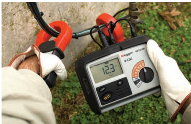
Model DET4TCR shown performing the stakeless ground testing method using only clamps.
