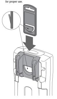
The universal hanger attaches to the meter and can be used by itself on a nail, hook, with a piece of rope or stiff wire.
