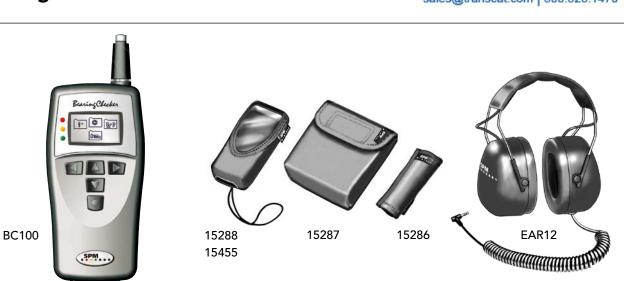
Bearing Checker is a portable instrument for fast and easy measurement of bearing condition in preventive maintenance. The instrument is push button controlled and basic measurement data are entered manually. Bearing Checker measures shock pulses with a built-in probe and machine surface temperature with an infrared sensor. The instrument can also be used as an electronic stethoscope for detecting machine sound irregularities.
