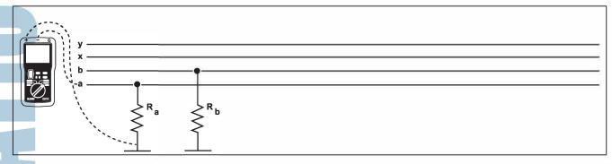
The results of the resistance measurement should be within +/- 20% of each other. Additionally the insulation resistance of each leg should be  $>50M\Omega$  to  $100M\Omega$ .
