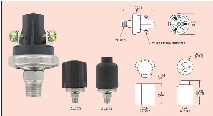
Series A6 Durable Pressure Switches have been specifically designed to stand up to extended duty applications. These switches are constructed with a polyimide film diaphragm and are compatible with a variety of fluids. For ease of installation, the switches come with a 1/4 male NPT process connection and can be mounted in any orientation. The Series A6 pressure switches are compact and have great setpoint integrity, and feature simple, easy set-point field adjustment.
