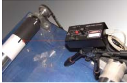
Tripod mounted SLS can provide TTL pulses from contrasting color targets.
