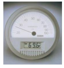
or adjustments. Analog humidity display; ½"H LCD temperature display. Supplied with one AA 1.5 V battery, corrosion-resistant plastic case, mounting bracket, and instructions.
